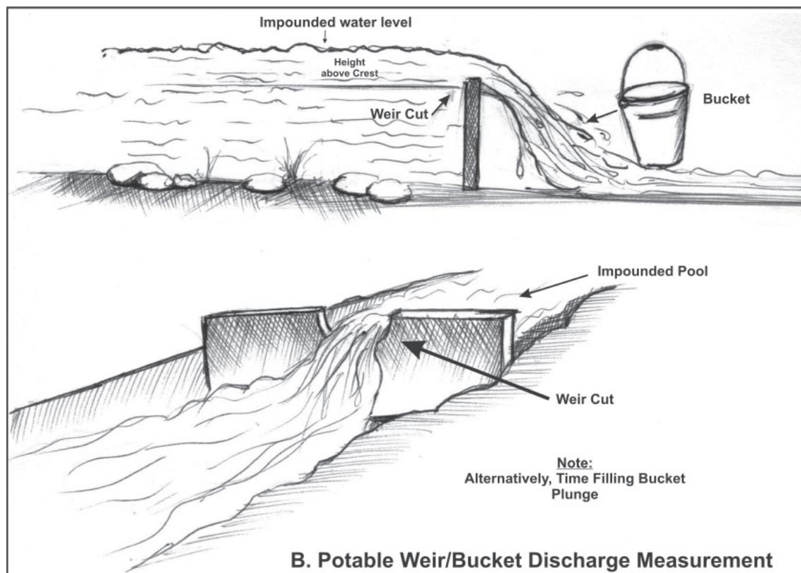
**B. Potable Weir/Bucket Discharge Measurement**
