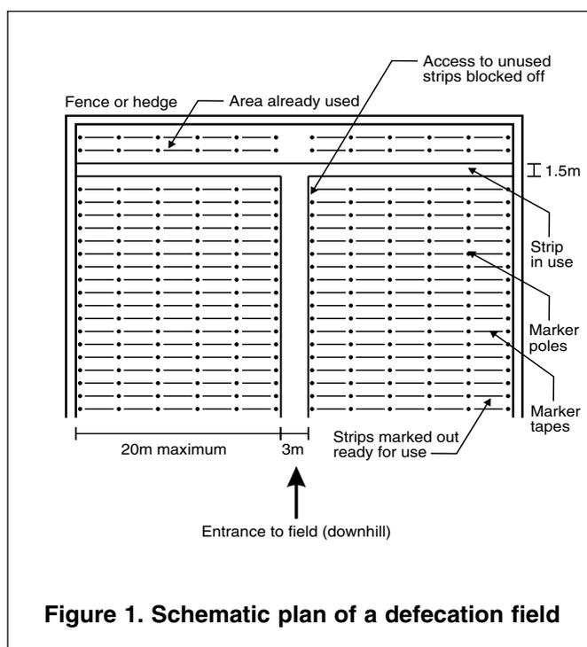
Figure 1. Schematic plan of a defecation field
