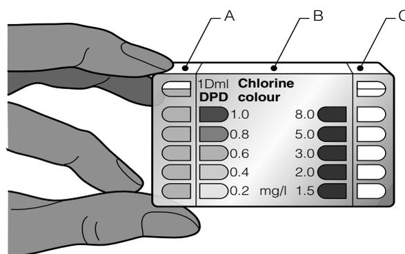
Note: A third chamber (C) would be used if a higher chlorine residual is to be measured.
