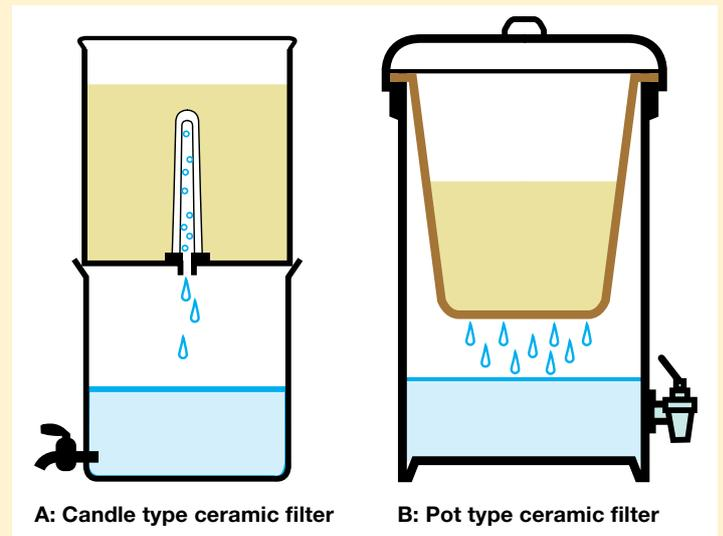
Generally, a porous ceramic filter sits on top of a plastic or metal receptacle, which is fitted with a tap. The ceramic filter material has tiny pores or microscopic holes specifically designed to trap small solid particles and pathogens, while letting water pass through slowly.
