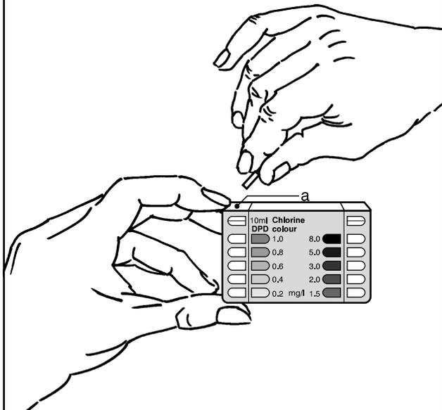
**Step 2.** Crush the tablet, then fill chamber (a) with the chlorinated water supply under test.
