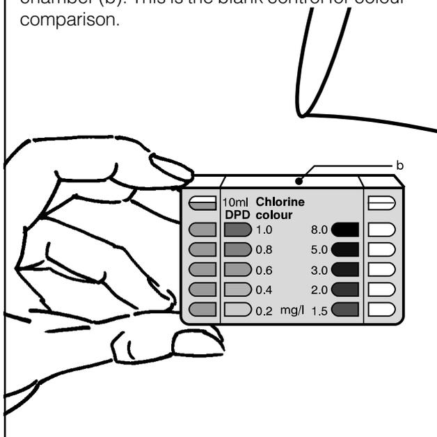
**Step 4.** The level of residual chlorine (R) in mg of chlorine per litre of water (mg/l) is determined by comparing the colour of the water supply under test in chamber (a) with the tablet added with the standard colours on the vessel (chamber (b)).
