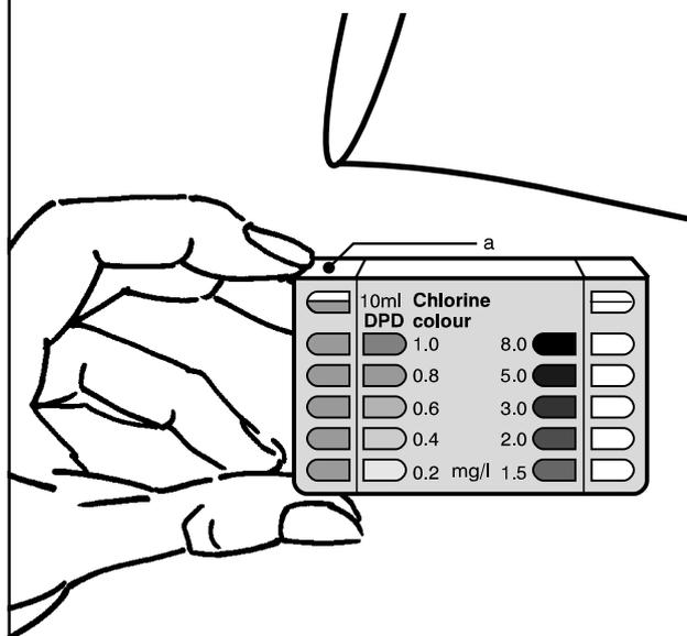
**Step 3.** Place more of the same water supply under test (without a tablet) in the second chamber (b). This is the blank control for colour comparison.
