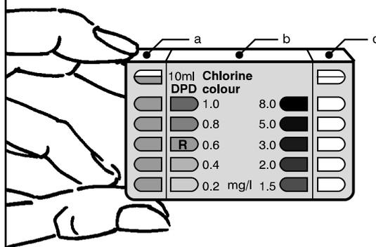
Note: Chamber (c) would be used if a higher chlorine residual is to be measured.
