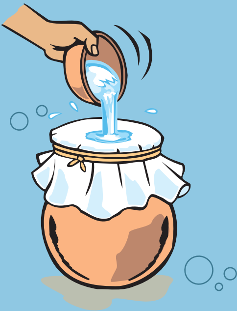
If water is not clear, filter the water using thick cotton cloth before you add the chlorine.
